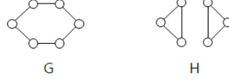
Figure 3: An example of a pair of non-isomorphic graphs that are not distinguishable by WL test.
