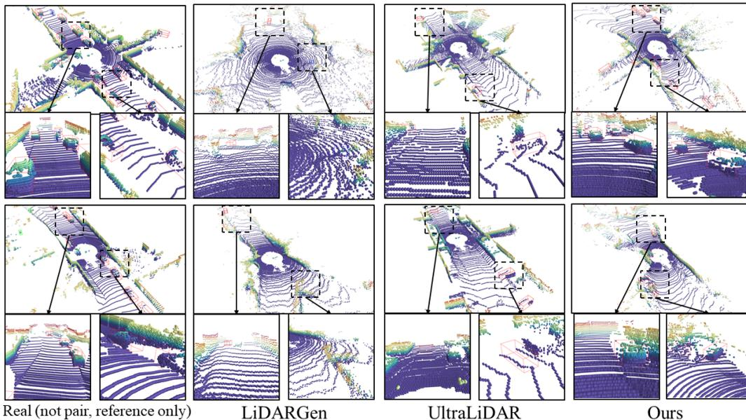
Figure 4: **Qualitative comparison against baselines on LiDAR generation.** We compare with LiDARGen, UltraLiDAR and include real LiDAR for reference. *OLiDM* generates LiDAR data with more realistic sparsity and beam patterns. Red, Blue and Green boxes are the detected objects (car, cyclist and pedestrian) from a 3D detector trained on KITTI.
