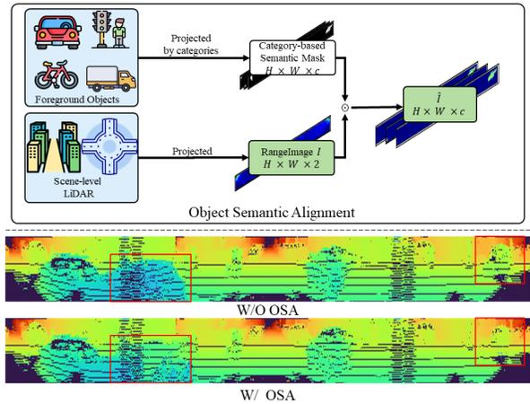
Figure 3: **The Object Semantic Alignment (OSA) module** aligns object features based on their semantic space, enhancing the foreground object generation and contributing to the overall quality of the generated LiDAR scenes.
