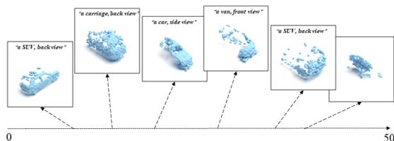
Figure 8: **Qualitative results about object-level generation on KITTI360.** *OLiDM* controls the generation of LiDAR objects with different 3D location and text prompts. The farther away an object is, the sparser the point clouds are.
