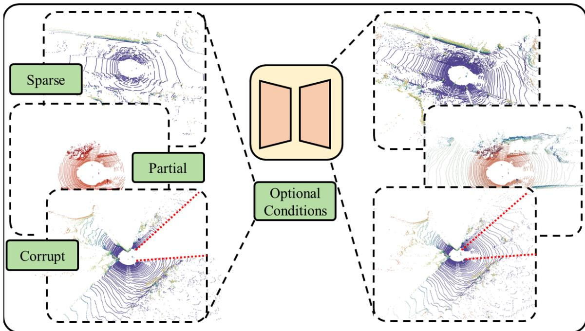
Figure 17: ***OLiDM* for conditional LiDAR scene generation.** *OLiDM* is capable of handling versatile conditions, achieving realistic and high-fidelity LiDAR data across various conditional generation tasks.
