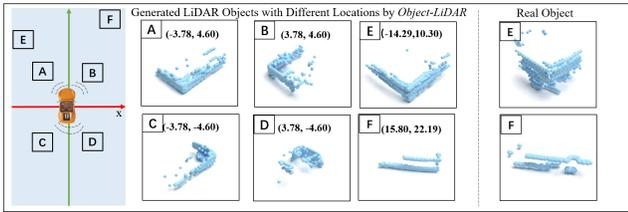
Figure 9: LiDAR scanning patterns vary across different 3D positions, as shown at locations A-F on the map. The first two columns images reveal symmetrical scanning patterns around a vehicle in four quadrants (A, B, C, D). *OLiDM* accurately mirrors real-world LiDAR scans at positions E and F, showcasing its ability to consistently replicate authentic scanning patterns across diverse spatial dimensions.
