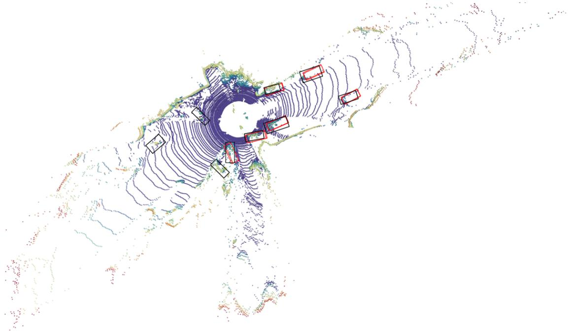
Figure 16: **Qualitative results about scene-level generation on KITTI-360.** *OLiDM* controls the generation of LiDAR scenes by conditioning foreground objects. **black** boxes indicate the given object locations as conditions while the **red** boxes are the detected ones on the generated LiDAR data.
