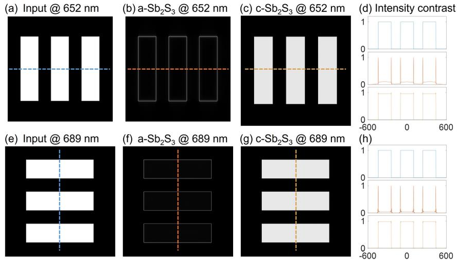
FIG. 4. Imaging results of a test chart and the corresponding horizontal/vertical intensity profiles at resonant wavelengths of 652 nm and 689 nm for amorphous and crystalline states.
