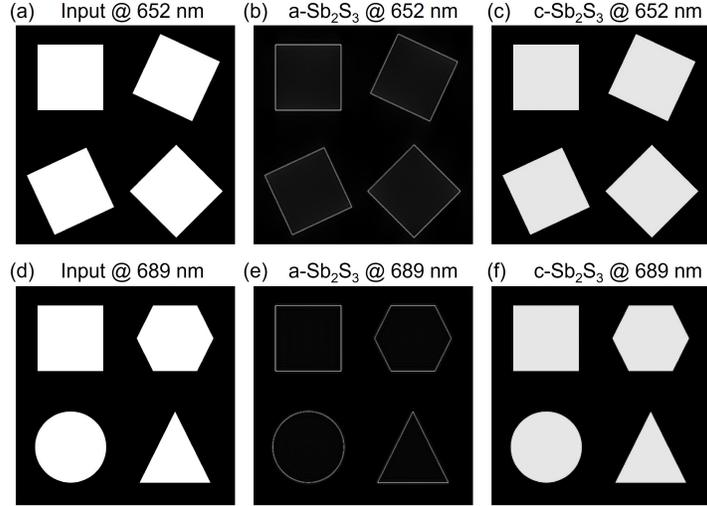
FIG. 5. Imaging results of different shapes at resonant wavelengths of 652 nm and 689 nm for amorphous and crystalline states.
