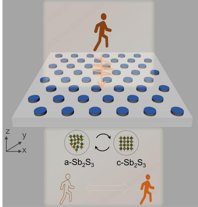
FIG. 1. Schematic of the Sb<sub>2</sub>S<sub>3</sub>-based metasurface for reconfigurable imaging processing. The functionalities of the metasurface are dynamically switched between edge-detection and bright-field imaging in the visible spectrum via adjusting phase states of nanostructured Sb<sub>2</sub>S<sub>3</sub> meta-atoms.
