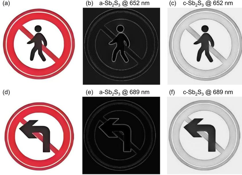
FIG. 6. Input and output images of two common traffic signs at resonant wavelengths of 652 nm and 689 nm for amorphous and crystalline states.
