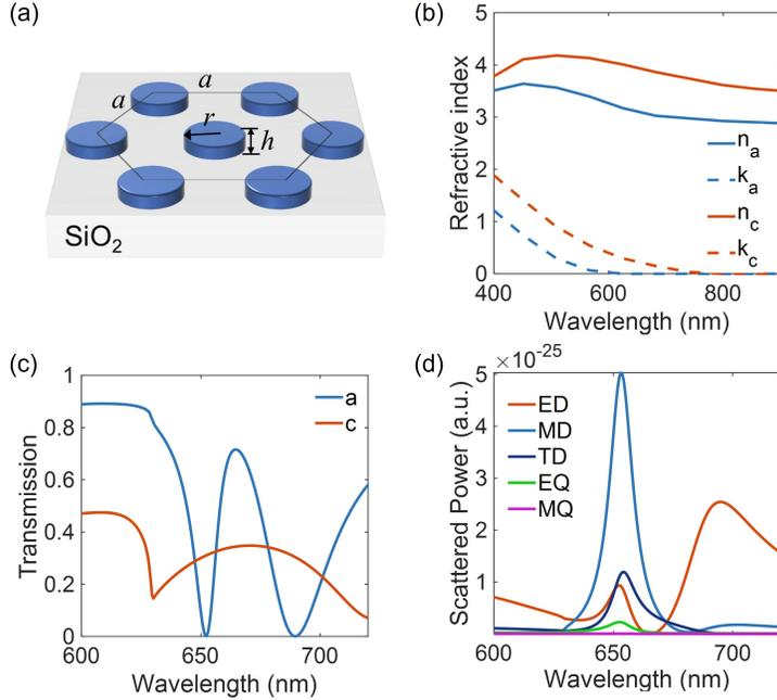
FIG. 2. (a) Schematic of a unit cell of the metasurface with optimized geometry of  $a=500$  nm,  $h=100$  nm, and  $r=160$  nm. (b) Refractive index of Sb<sub>2</sub>S<sub>3</sub> in the amorphous and crystalline states. (c) Simulated transmission spectra under normal incidence for both states. (d) Results of multipolar decomposition for amorphous state.
