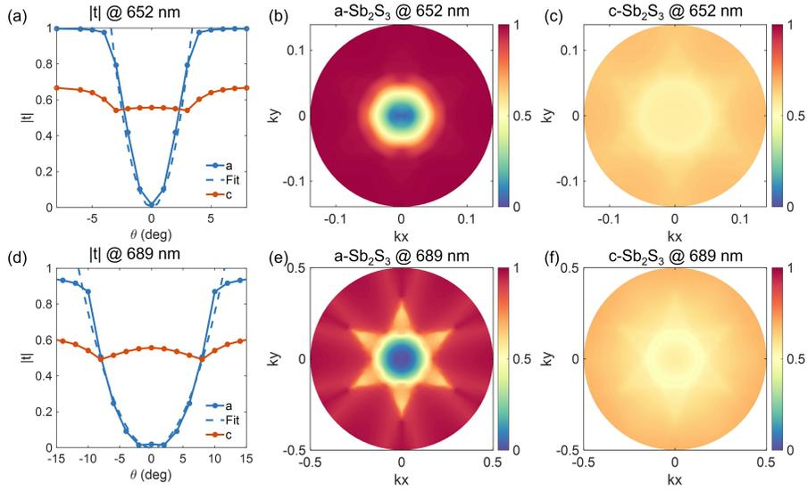
FIG. 3. Angular dispersion of the metasurface at resonant wavelengths of 652 nm and 689 nm for amorphous and crystalline states under  $x$ -polarization incidence. (a)(d) Transmission amplitude as a function of incident angle. (b)(c)(e)(f) The results of optical transfer functions.
