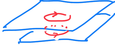
FIG. 2. Chiral electronic double layer: circular edges create counterflowing currents.
