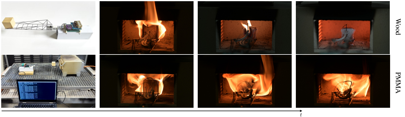
Figure 7: Experimental setup for mass loss and temperature measurement. Samples of different materials (wood and PMMA) are equipped with thermo probes and placed on a scale arm inside an oven that heats the sample up until the ignition temperature. During the combustion process, the weight and temperature and different depths (surface, sub-surface, and core) are continuously recorded.
