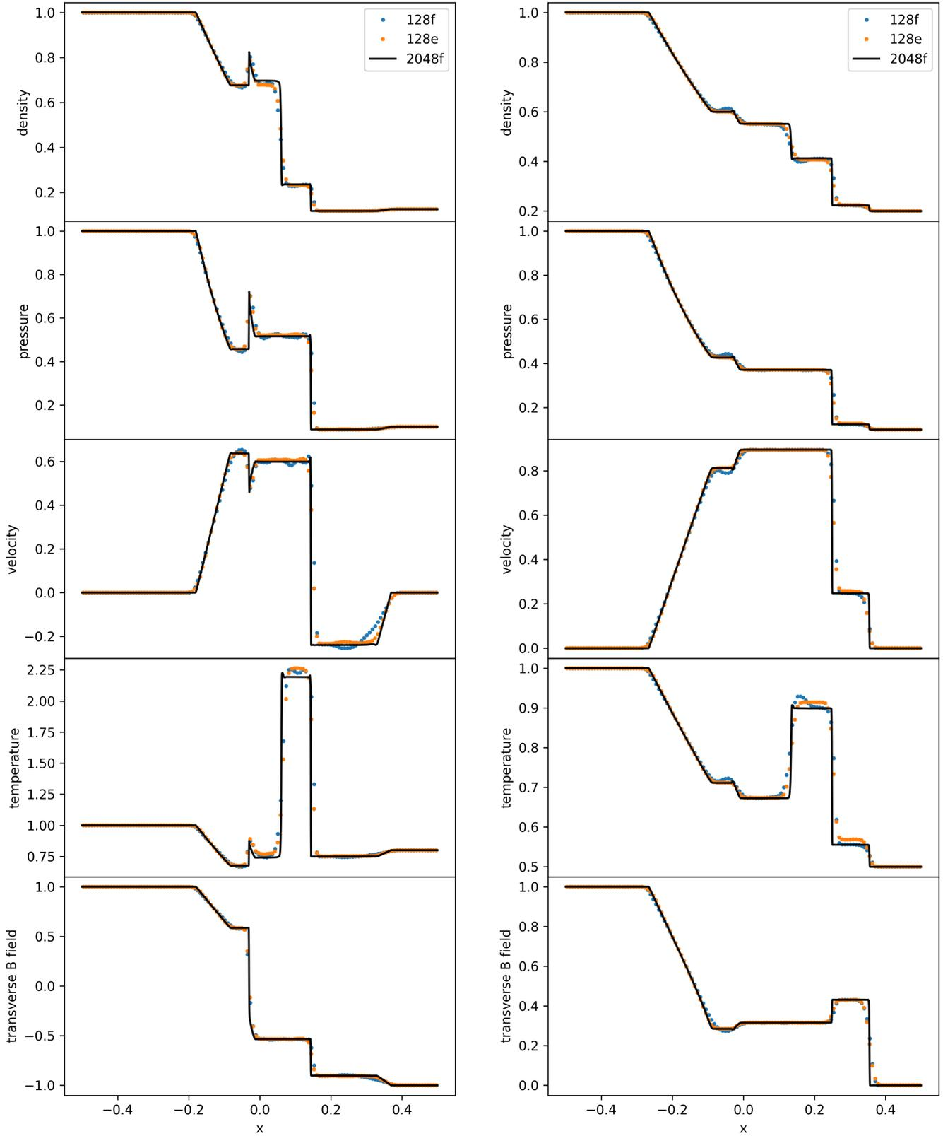
**Figure 2.** *Left:* Density, pressure, velocity, temperature, and transverse field for the Brio & Wu (1988) test at  $t = 0.2$ . *Right:* Same quantities for the switch-on shock test (Balsara 1998). Black lines indicate the reference solution on a fixed grid with 2048 cells. Blue symbols denote the fixed grid solution at 128 cells, and orange ones the co-scaling grid solution, also at 128 cells. Over- and undershoots appearing in the fixed-grid solution are reduced for the co-scaling grid.
