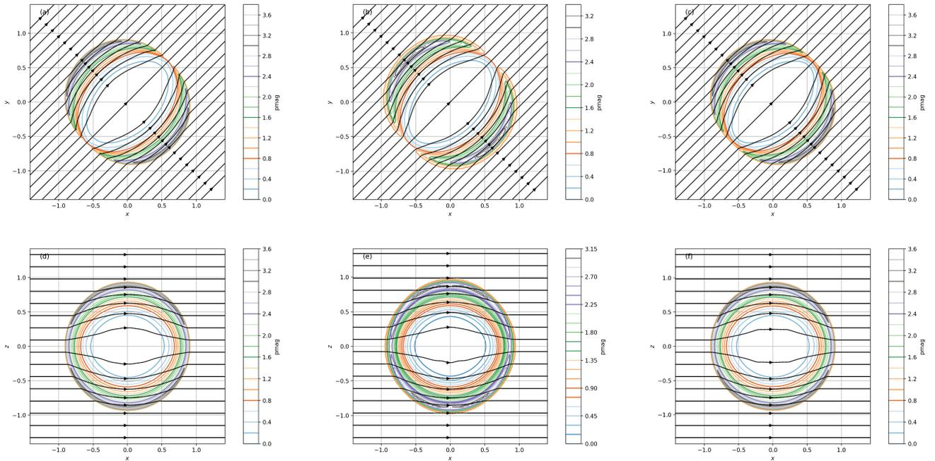
**Figure 6.** Midplane slices in magnetic pressure  $B^2/2$  for the three-dimensional blast test. Shown are slices in the  $(x, y)$ -plane (top row) and  $(x, z)$ -plane (bottom row). (a,d) Fixed grid at  $512^2$ , (b,e) co-scaling grid at  $128^2$ , (c,f) co-scaling grid at  $512^2$ . Color lines indicate 20 equidistant contours in magnetic pressure between 0 and 3.7. Streamlines have been overplotted in black.
