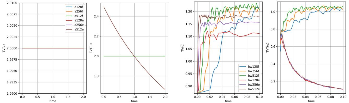
**Figure 7.** TV (first and third panel) and TOTV (second and fourth panel) measured in the density for the advection test (see text) and the Brio-Wu test (Sec. 4.1). Models with a trailing  $f$  use a fixed grid, and models with a trailing  $e$  use the co-scaling grid. Numbers indicate numerical resolution. Both fixed and expanding grid are TVD and TOTVD. For the Brio-Wu test, TVD is not expected initially, since the initial conditions lead to shocks and thus additional structure.
