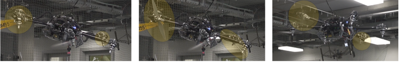
Fig. 13: From left to right: the Aerial Robot is hovering in place, then the propellers are commanded to stop and the arms to rotate. Finally the propellers are enabled again and the arms slowly align with gravity again to balance the actuators' usage. The stopped propellers are highlighted in yellow.
