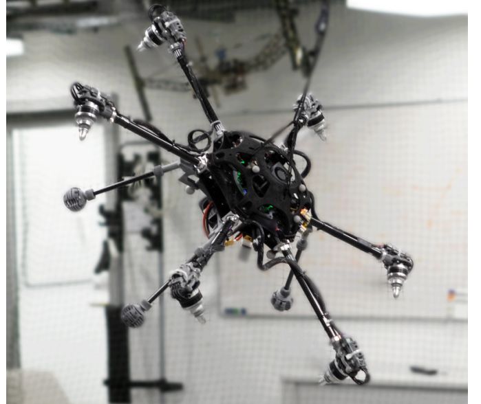
Fig. 1: The Omnidirectional Aerial Robot hovering at a tilted configuration. All the experiments are executed on this platform.
