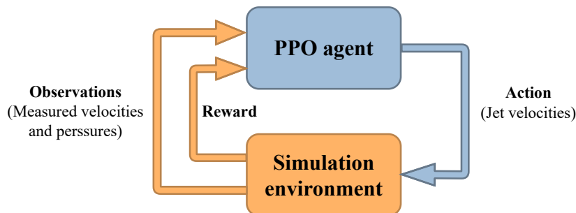
FIG. 3. Schematic of the PPO agent closed-loop control.
