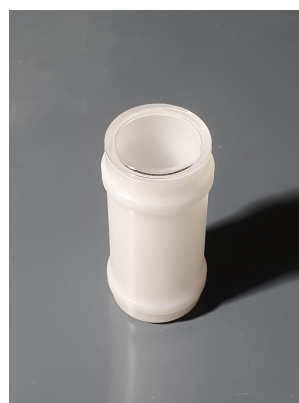
Figure 4. Picture of the floating gauge. It is made of PTFE for its density and chemical properties. A quartz glass window is glued on one end of the tube with epoxy glue.
