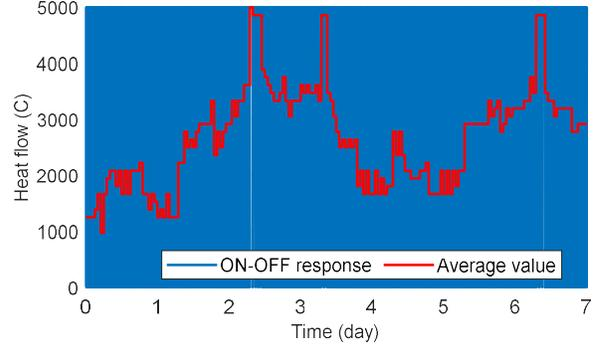
Fig. 5. The heat power consumption in switching waveform and average.
