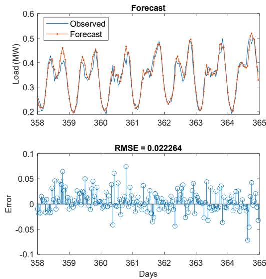
Fig. 13. The one time-step (1 hour) forecasting performance on the last week.
