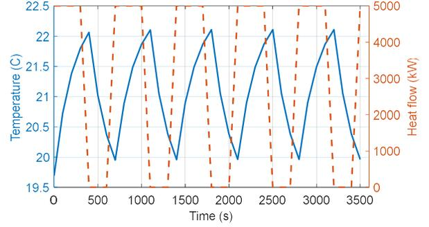
Fig. 2. Indoor temperature response under the switching heat flow.
