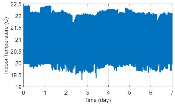
Fig. 4. Indoor temperature response with the close-loop control of the relay-based ON-OFF controller.
