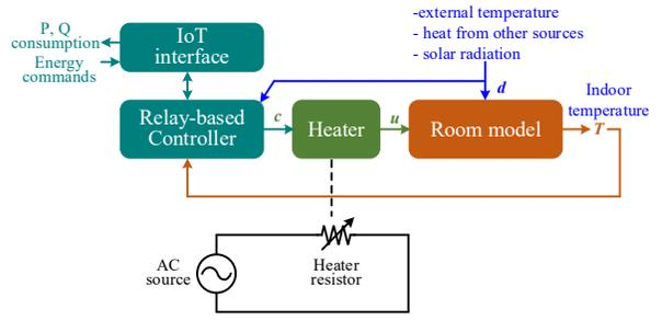
Fig. 1. Block diagram of IoT-based thermostatic load model.
