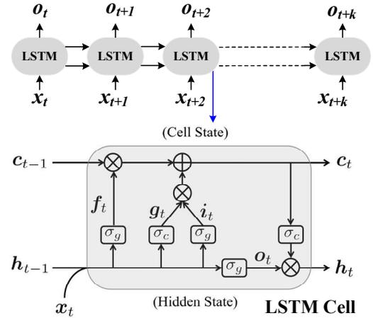
Fig. 6. The general structure of an RNN with LSTM cell.
