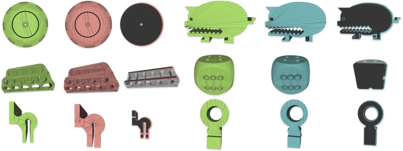
Fig. 12. Our approach supports the generation of feature-preserving non-uniform offsets, i.e. from 0.01l to 2l for each model, for any given mesh inputs (green), either inwardly (cyan) or outwardly (red).
