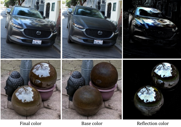
Figure 3. Visualization of reflection and base color. Our method successfully reconstructs near-field and distant reflections using the environment Gaussian instead of baking into the base color.
