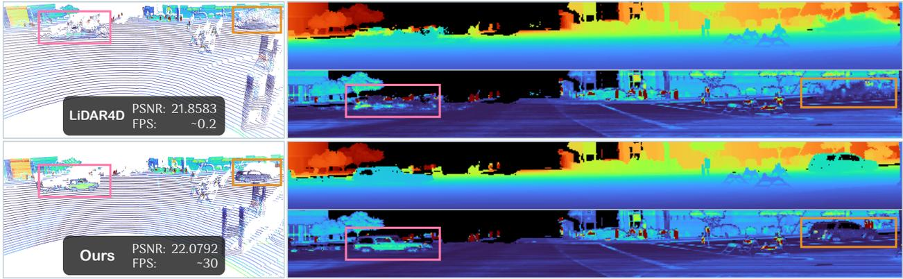
Figure 1. **Realistic and real-time rendering of LiDAR view in dynamic driving scenes.** Our LiDAR-RT produces high-fidelity LiDAR view at 30 FPS (64×2650) within 2 hours of training. SOTA method [58] struggles to model the dynamic objects in complex scenes and suffers from high training and rendering costs (15 hours for training and 0.2 FPS for rendering a range image).
