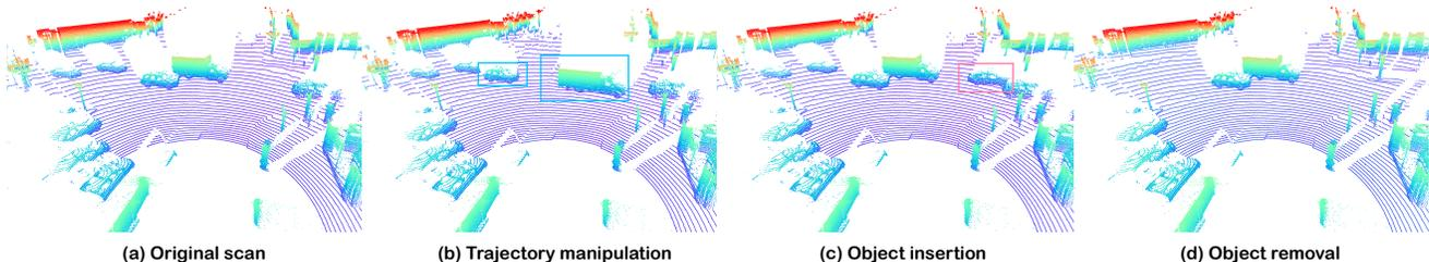
Figure 5. **Scene editing results on the Waymo dataset [40].** Our method supports various scene editing operations, including trajectory manipulation, object insertion, and object removal. The boxes ( $\square/\square$ ) highlight the edited objects.
