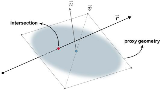
Figure 3. **Ray intersection with proxy geometries.** We construct the proxy geometry for each 2D Gaussian primitive as a pair of co-planar triangles, then the ray tracer performs intersection tests with the vertices  $\vec{v}$  and surface normal  $\vec{n}$ .
