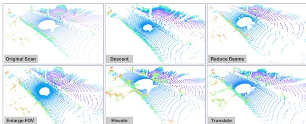
Figure 6. **LiDAR re-simulation results with different sensor configurations on the Waymo dataset [40].** Our LiDAR-RT can generate realistic LiDAR point clouds with varying sensor poses, beam numbers, and FOV settings.
