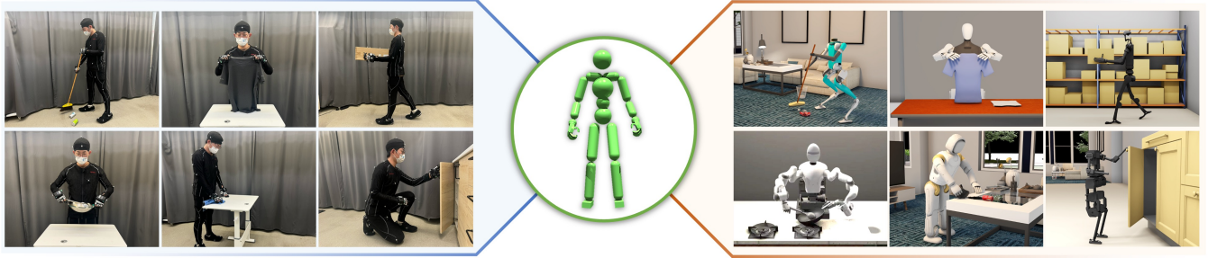
Fig. 1: Human can serve as the prototype of diverse humanoid robots, efficiently learning generalized loco-manipulation skills without considering configuration differences. The framework introduces a unified digital human (UDH) model (the green humanoid) to aggregate human behaviors from embodiment demonstrations. Loco-manipulation skills are generated by combining behavior primitives through adversarial imitation, and subsequently deployed on diverse humanoid robots using efficient motion retargeting and fine-tuning techniques.
