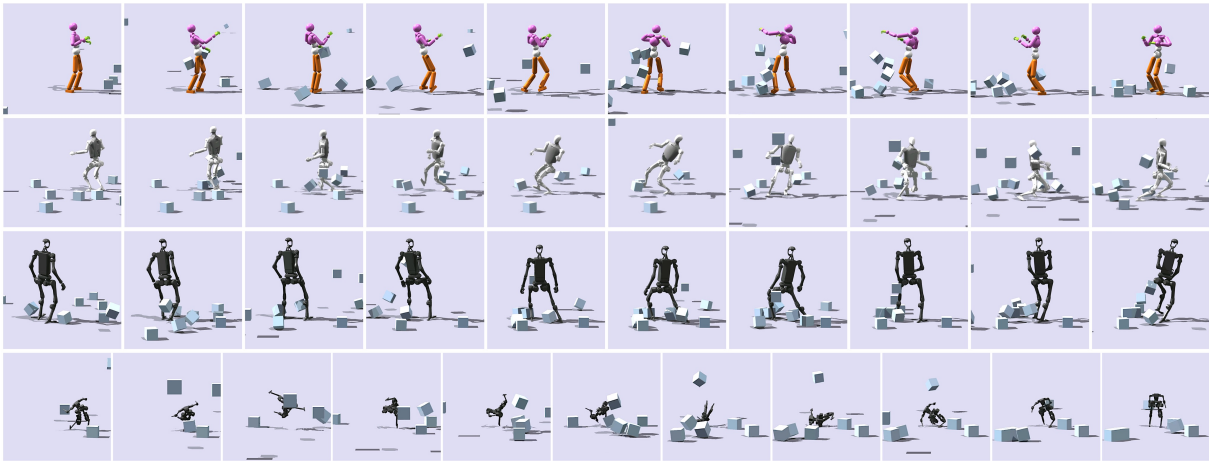
Fig. 6: Behavior primitive pre-training. Stability experiments for legged humanoid robots by hitting them with moving cubes.
