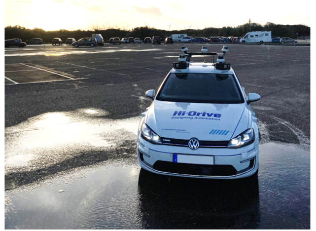
Fig. 3: The test vehicle, a Volkswagen E-Golf equipped with experimental automation
