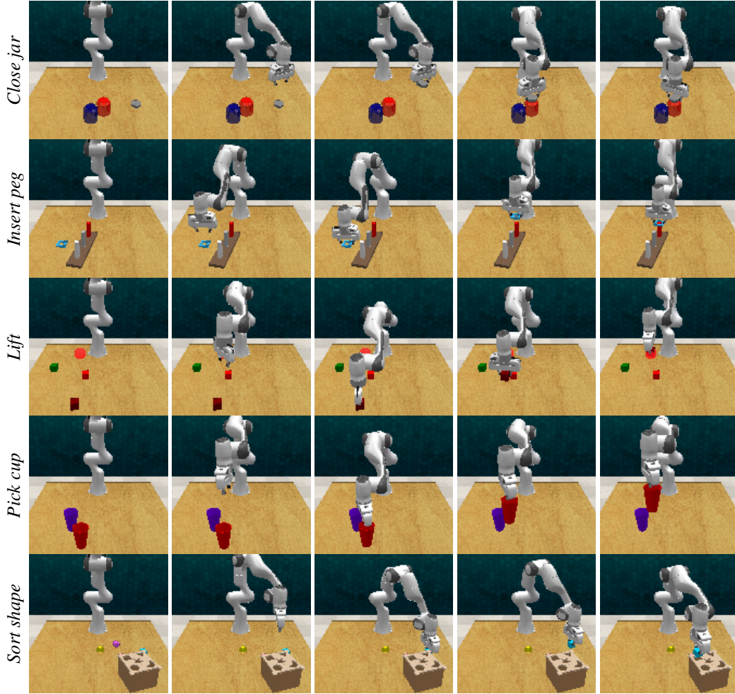
Figure F.7: Visualization of the simulation tasks. From top to bottom: close jar , insert peg , lift , pick cup , sort shape
