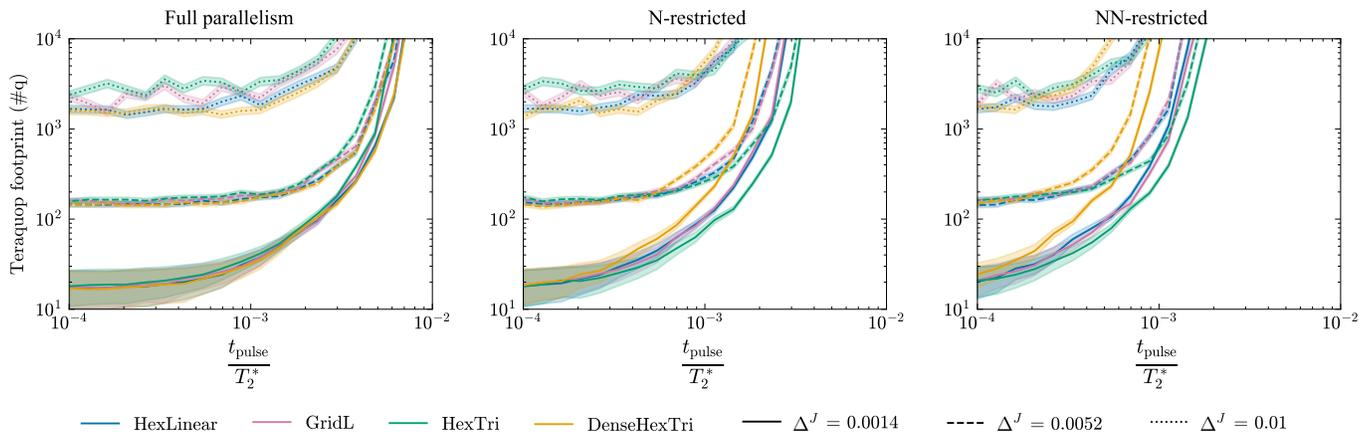
FIG. 11. Teraquop footprints for all four layouts, under different parallelism conditions and in different noise regimes. The ratio  $\frac{t_{\text{pulse}}}{T_2^*}$  varies along the x axis and each plot contains three groups of lines corresponding to different  $\Delta^J$  strengths.
