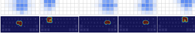
Fig. 8: Keystroke heatmap generation when the VR user types the word “HELLO” on the virtual keyboard. Upper part: confusion matrices of extracted IR features. Lower part: generated heatmaps on the virtual keyboard (§ IV-D).
