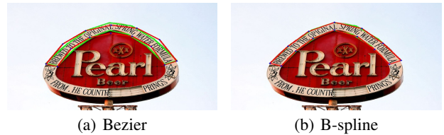
Figure 7: Visualization comparison of different interpolation methods. The green polygons are ground-truth and the red lines are interpolated curves.
