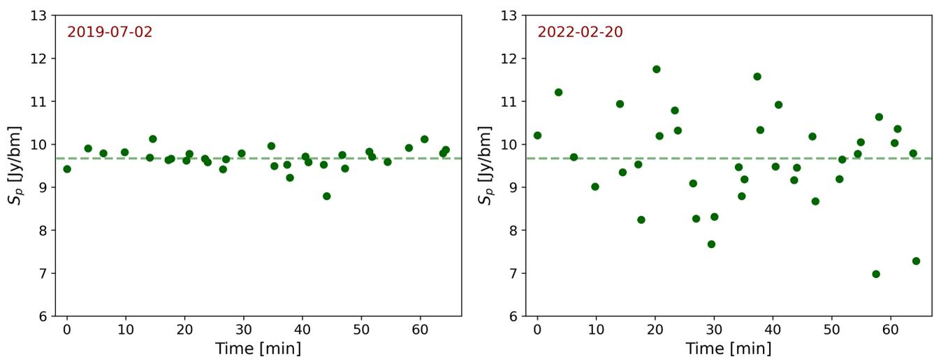
**Figure 11.** Calibrated VCSS light curves for the compact source PKS 2135-20. Left: observation on 2019-07-02, when the source was  $140^\circ$  from the Sun, shows a steady light curve. Right: observation on 2022-02-20, when the source was  $13^\circ$  from the Sun, reveals strong scintillations. Dashed lines indicate the average brightness from 2019-07-02. Measurement uncertainties are smaller than the plotted markers.
