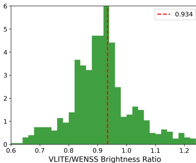
**Figure 3.** Histogram of the brightness ratios of unresolved WENSS sources detected within  $8'$  of the VLITE primary beam center. The weighted average of 0.934 sets the normalization of the primary beam.
