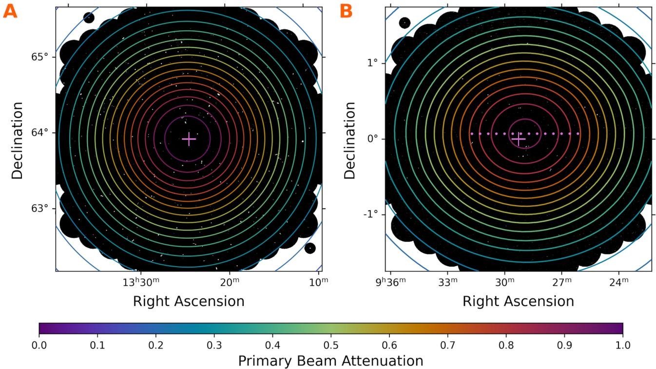
**Figure 6.** Contours of primary beam attenuation overlain on  $3.5^\circ$  wide B configuration images. **(A)** A standard VLITE image. **(B)** A VCSS snapshot image. The on-the-fly observing mode smears the VLITE primary beam by  $1.5^\circ$  in right ascension, producing an elongated attenuation pattern offset from the pointing center. Points indicate the beam center sampling during the smear.
