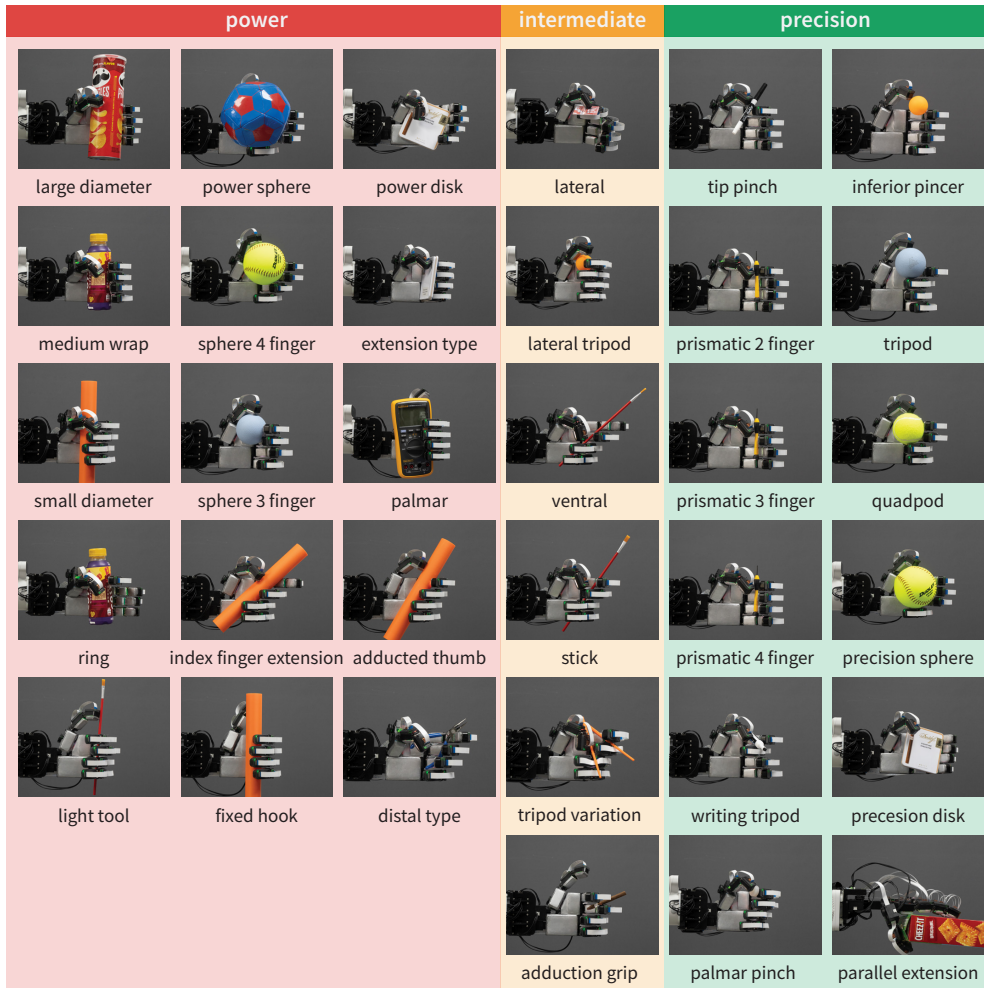
Fig. 3 | Workspace of the F-TAC Hand. Empowered by its smart design, the workspace of the F-TAC Hand enables it to perform all 33 human grasping types, as documented by Feix et al. [23].
