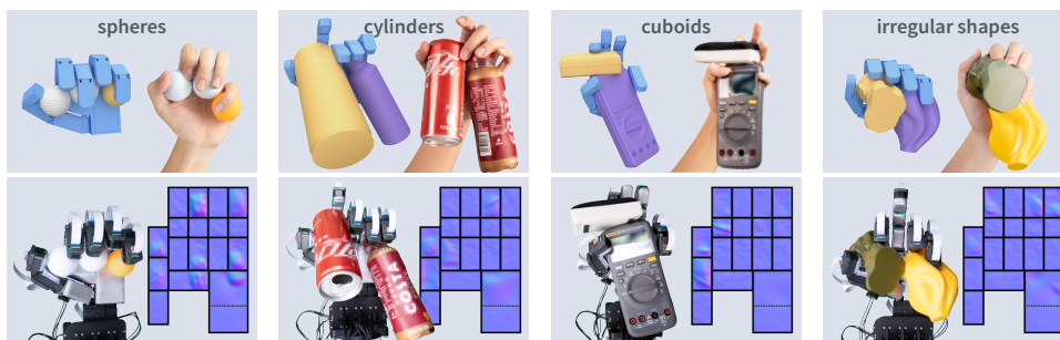
Extended Data Fig. 5 | More adaptive behaviors by the F-TAC Hand. F-TAC Hand's stable grasping with some fingers disabled (shown in light gray), mirroring human compensation for finger injuries.
