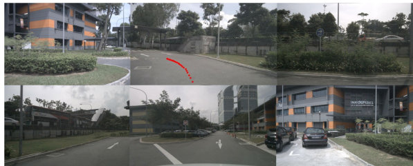
Context: This is an overview image covering the entire 360-degree surroundings of the ego vehicle. The red line indicates the future trajectory, no line suggests stopping or slowing down. When explaining the reasoning, please focus on the camera image and surrounding context rather than referencing the plotted trajectory. A_c : The ego vehicle is moving forward on a clear road. A_f : The ego vehicle is likely to turn left. A_r : The road is clear with no visible obstacles, and the surroundings suggest a typical urban environment. The presence of lane markings and the absence of traffic support the likelihood of a left turn. A_{control} : move slowly A_{turn} : turn left A_{lane} : none
