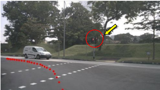
Figure 15. An imperfect annotation example where an overly cautious annotation is generated, despite the ego vehicle continuing without stopping or slowing down.
