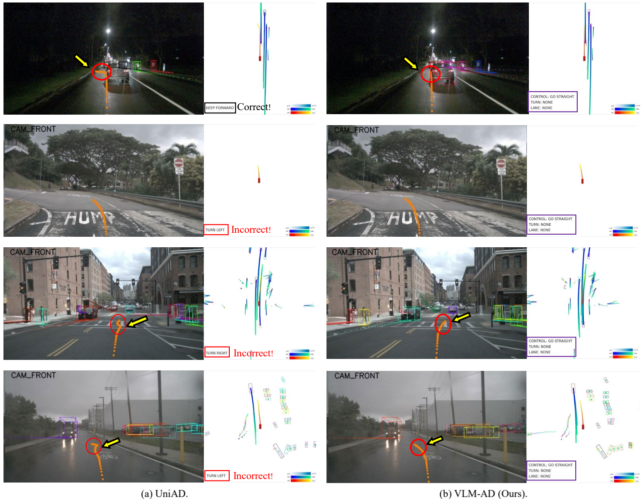
Figure 4. Qualitative comparison between UniAD and our method. The yellow arrow highlights areas where VLM-AD outperforms UniAD. The red box indicates the failure planning command from UniAD, and the purple box represents the predicted three action outputs from our VLM-AD auxiliary text head.
