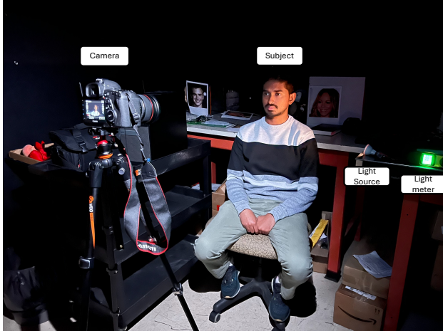
Figure 8. (Left) Environmental setup, real-life low-light noisy photo taken in the dark room. (Right) Visual comparison on the real-world captured SUBJECT.
