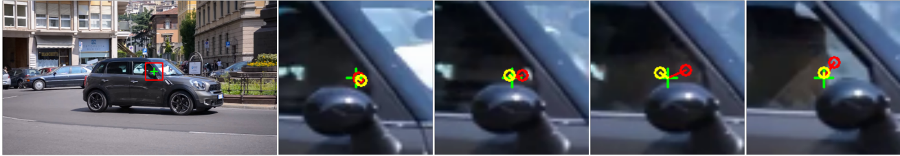
Figure 5. Qualitative results obtained by TRecViT for point tracking on DAVIS dataset compared to VideoMAE. The leftmost image indicates the point to track in the original frame, and the images towards the right show zoom-ins on subsequent frames. Green plus (+) marker indicates the ground truth, yellow circle indicates TRecViT’s predictions and red circles indicate VideoMAE’s predictions.
