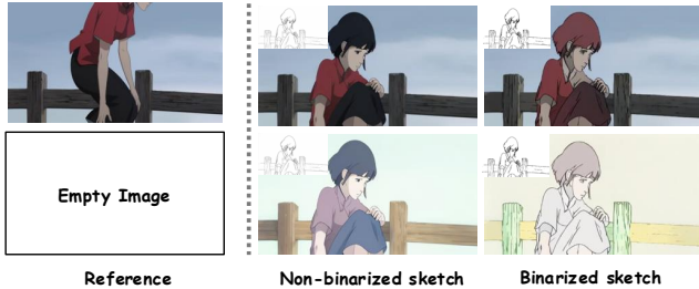
Figure 4. Illustration of color leakage issue in non-binarized sketch. For previous video colorization method [21], when given non-binarized sketch, even if the reference is an empty image, it can still generate colorized results with similar color pattern to the ground truth. After binarizing the sketch, the colorization results degrade significantly.
