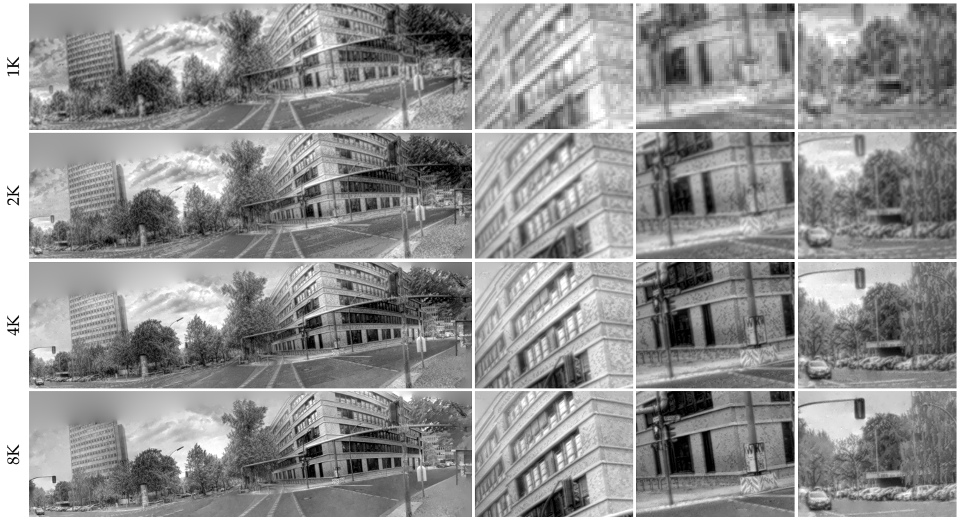
Fig. 13: Results of running EPBA at several map resolutions, from 1K ( 1024 \times 512 px) to 8K ( 8192 \times 4096 px). The intensity maps are recovered from scratch (zeros), and the initial rotations are provided by IMU dead-reckoning. The insets have a width of 500 px at the 8K scale.
