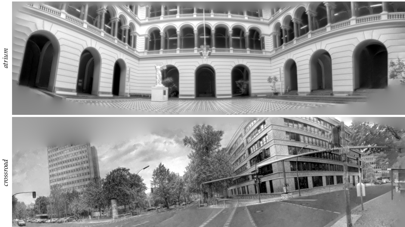
Fig. 11: Results of EPBA in the wild (without ground truth). The intensity maps are recovered from scratch (zeros). (a) atrium is recorded by a Prophesee EVK4 (1 Mpixel camera), where initial rotations are provided by CMax- \omega angular velocity integration. Crop from a 4096 \times 2048 px map. (b) crossroad is recorded using a DVXplorer (VGA resolution), and initial rotations are provided by IMU angular velocity integration. Crop from an 8192 \times 4096 px map.
