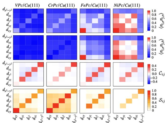
**Figure 5.** Heat-map representations of the (a) double occupation  $\langle n_{i,\sigma} n_{j,\sigma} \rangle$  for like spins, (b) double occupation  $\langle n_{i,\sigma} n_{j,\bar{\sigma}} \rangle$  for opposite spins, (c) charge- and (d) spin-fluctuation as defined in eqs 5 and 6.
