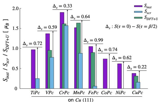
**Figure 3.** Dynamical screening of the effective moments in TMPc molecules on Cu(111). Unscreened (purple), screened (cyan), and DFT+U effective local moments (green) for TMPc molecules on Cu(111).  $\Delta_s$  is the difference between the instantaneous and the screened spin moments.
