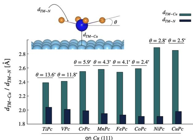
**Figure 1.** Structural details of the adsorbed transition-metal phthalocyanine molecules on the Cu(111) surface.  $d_{TM-Cu}$  and  $d_{TM-N}$  represent the closest distances between TM and surface Cu layer and intramolecular axial bonds between TM and N atoms, respectively.  $\theta$  quantifies the degree of nonplanarity in the adsorbed molecules.
