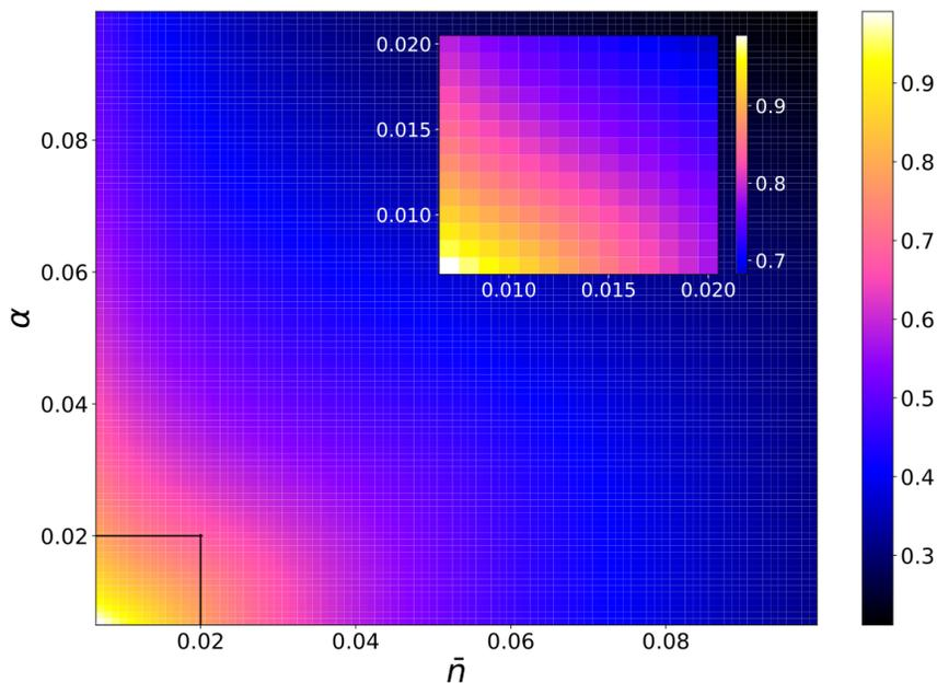
**Figure 4.** Simulation of the visibility of a HOM experiment between independent photons as a function of their emission parameters,  $\alpha$  and  $\bar{n}$ . *Inset:* zoom on the zone for which  $\bar{n}$  and  $\alpha$  are below 0.02, corresponding to a visibility above 70%.
