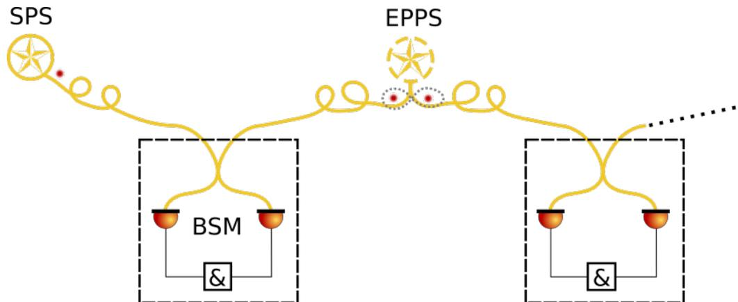
**Figure 1.** Simple schematic of a quantum network operation for long distance propagation, using a single-photon source (SPS), an entangled photon-pair source (EPPS), and a Bell state measurement (BSM) apparatus.
