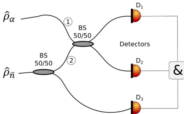
**Figure 2.** Model-scheme experiment. The coherent state interferes with one member of a photon pair. The separation of paired photons and the combination of the interfering are ensured by beam splitter (BS) operation. Then, detection is performed ( $D_{1-3}$ ) and heralded two-fold coincidences are recorded ( $\&$ ). 1 and 2 represent the impinging modes at the BS responsible for the HOM interference.
