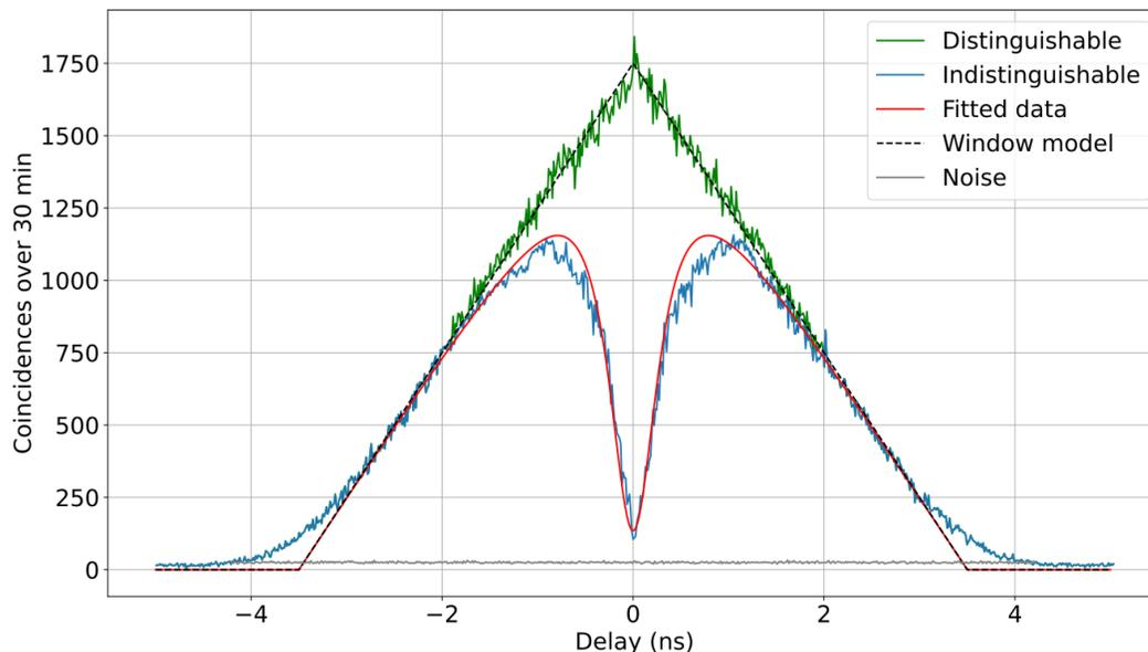
**Figure 6.** Coincidence histograms recorded during 30 min as a function of temporal delay,  $\tau$ , between SNSPDs. *Green curve:* data when photons are maximally distinguishable ( $\Delta\nu = 6\text{ GHz}$ ); *blue curve:* data when photons are maximally indistinguishable  $\Delta\nu = 0\text{ GHz}$ ); *red curve:* fit based on experimental properties; *grey curve:* total noise; *dashed black line:* temporal window of the coincidence histogram.
