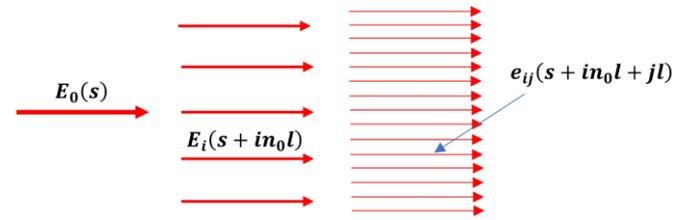
**Figure 4.** The scheme of laser illumination transformation along the optical path during its propagation through the illumination system with a passive speckle reduction method.
