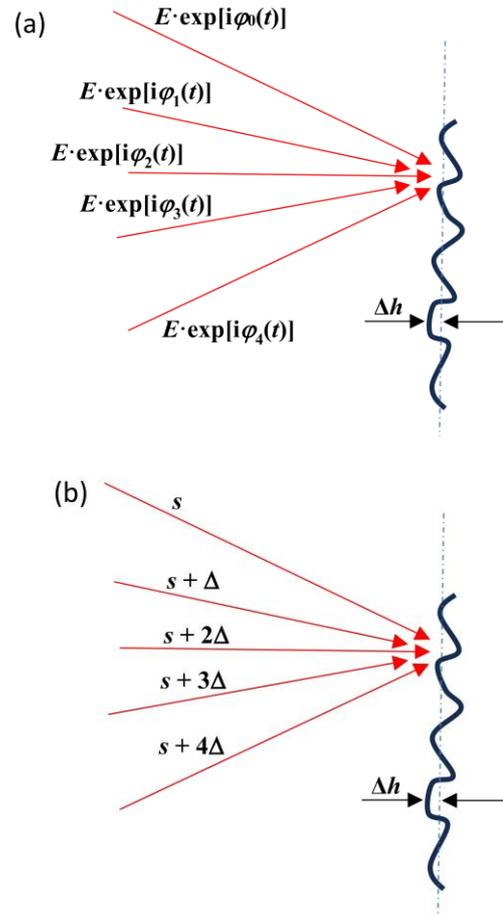
**Figure 3.** Schematic of the light scattering on a screen by sub-beams at angles decorrelated for speckle patterns for (a) the active sub-beam decorrelation method:  $\langle \exp[i\phi_n(t)] \exp[i\phi_m(t)] \rangle = \delta_{nm}$  – averaging over the integration time of intensity in the eye, where  $\delta_{nm}$  is the Kronecker delta; and (b) the passive method.
