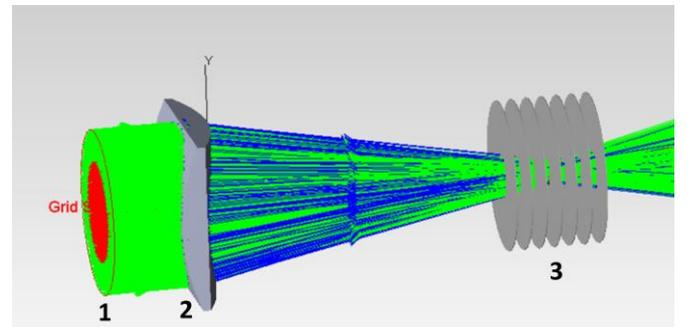
**Figure 9.** Simulation of light intensity distribution using the Monte Carlo ray-tracing method: 1 – Grid light source, 2 – the lens, and 3 – a set of fully transparent monitors.
