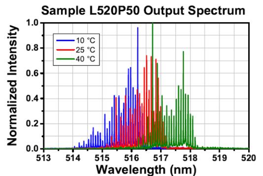
**Figure 13.** Light spectrum of the L520P50 laser diode (LD) at different temperatures [31].
