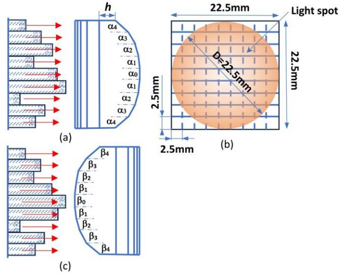
**Figure 6.** Optical system comprising two 1D cylindrical Fresnel lenses with a continuous surface profile and a 2D array of rectangular prisms of varying heights, designed for decoherent focusing of illumination into a rectangular light spot. (a) Top view; (b) Front view showing the light spot (orange circular spot); (c) Side view. Red arrows indicate the light rays.
