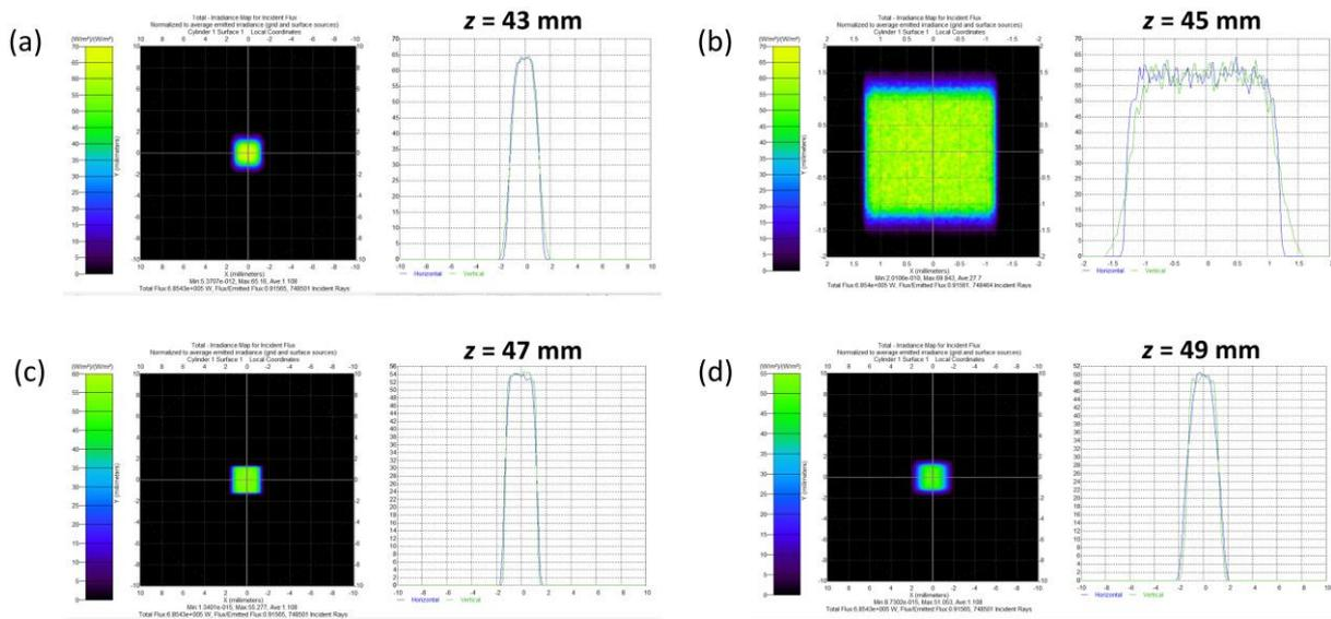
**Figure 11.** Intensity distribution of a Gaussian laser beam (clipped at the level of focus by Lens 2) at various distances from the lens: (b)–(d) show the transverse intensity distribution within the beam at different distances  $z$ .
