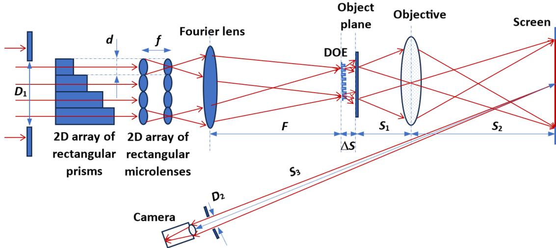
**Figure 12.** The optical setup used to evaluate the effectiveness of the speckle reduction method. Parameters:  $D_1 = 4$  mm,  $d = 0.4$  mm,  $f = 10$  mm,  $F = 240$  mm,  $\Delta S = 3$  mm,  $S_1 = 65$  mm,  $S_2 = 185$  mm,  $S_3 = 870$  mm,  $D_2 = 1$  mm.
