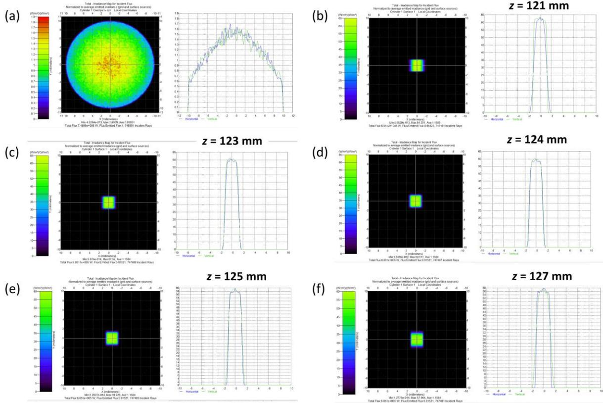
**Figure 10.** Intensity distribution of a laser beam focused by Lens 1 at different distances from the lens: (a) Initial Gaussian intensity distribution obtained in the model with the periphery truncated at the  $1/e$  level by an aperture; (b)–(f) Transverse intensity distribution of the beam at various distances  $z$  from the lens.
