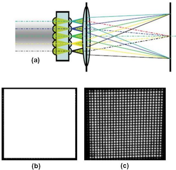
**Figure 1.** (a) Optical system for uniform illumination without significant optical energy loss; (b) optical spot under incoherent illumination; (c) optical spot under laser illumination. Reprinted from [8].
