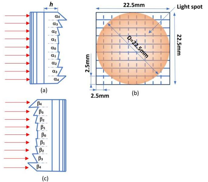
**Figure 7.** Optical system featuring two 1D Fresnel lenses in a planar configuration with a sawtooth surface profile, designed to focus illumination into a rectangular light spot using a 2D prism array. (a) Top view; (b) Front view showing the light spot (orange circle); (c) Side view. Red arrows indicate light rays.
