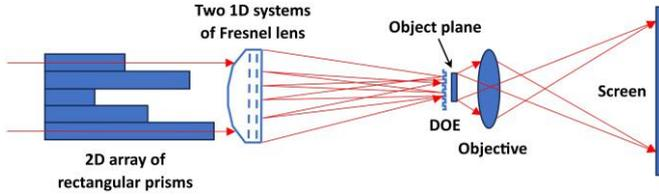
**Figure 5.** The principal optical scheme of the proposed illumination system.
