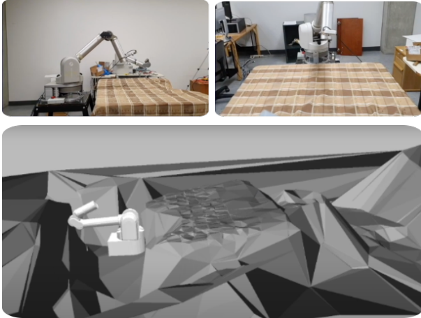
Fig. 3: Monocular surface mesh reconstruction using semi-dense CARV of the remote environment.
