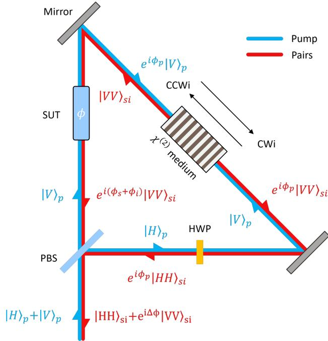
FIG. 1. Principle of a non-linear Sagnac interferometer in free space configuration using a type-0 phase matched medium. The blue (red) path represents the propagation of the pump (pairs). HWP: half-wave plate; PBS: polarizing beam splitter; CWi: clockwise; CCWi: counter-clockwise; SUT: sample under test.
