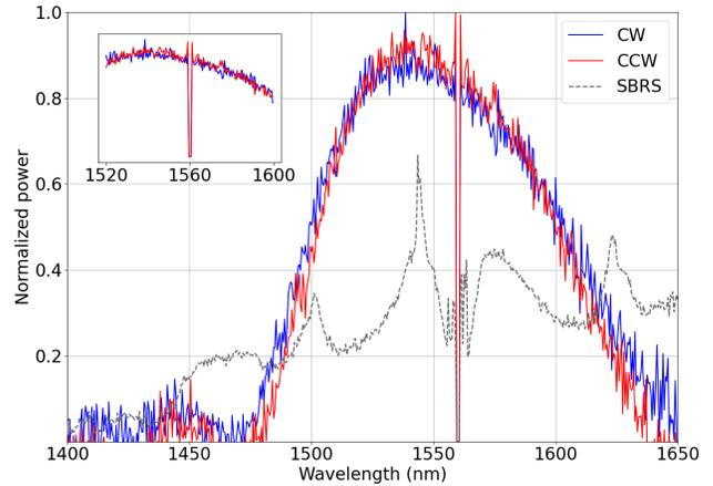
FIG. 3. Spectrum of the photon pairs measured by inserting an optical spectrum analyser inside the Sagnac loop. The blue curve represents the spectrum in the CWi path, while the red curve represents the spectrum in the CCWi path. The inset provides a closer view of the measurement area. The grey dotted line corresponds to the Spontaneous Raman Back Scattering (SBRS) spectrum. The dip around 1560 nm corresponds to the wavelength-division multiplexers (WDMs) used to filter out the residual pump.
