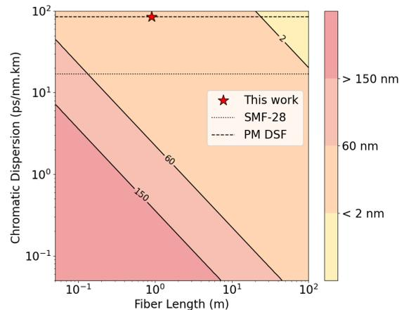
FIG. 5. Spectral width of the first quadratic two-photon fringe as a function of the sample length and its CD value. The dotted lines represent the dispersion value of the SUT and a standard SMF-28 telecom fiber. PM DSF: polarization maintaining dispersion-shifted fiber.
