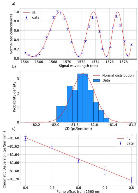
FIG. 4. a) Normalized coincidence measurement as a function of the signal wavelength, the blue dots are fitted using Eq. 10. b) Histogram of extracted CD for 100 measurements at  $\lambda_p = 1560.800$  nm. The red line is calculated assuming a normal distribution. c) Extracted CD for different pump wavelengths. The red curve represents a linear fit used to extract the TOD.
