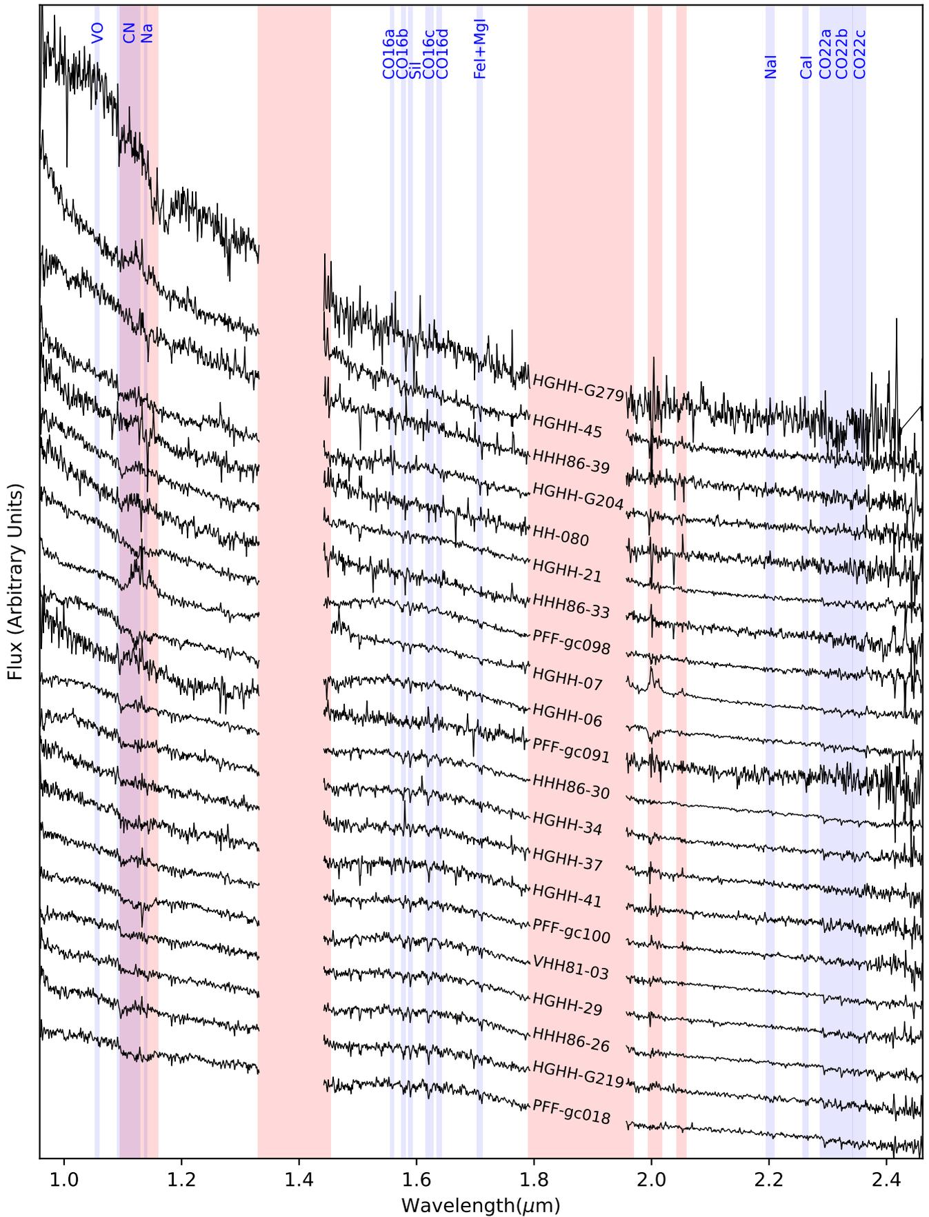
**Fig. 2.** NIR spectra of our sample, normalized at the H band plus a constant, and sorted by J-K colour. Regions with high telluric absorption are masked in red. We also highlight in blue the main stellar absorptions from Riffel et al. (2019) with a sufficient S/N and without an optical counterpart.
