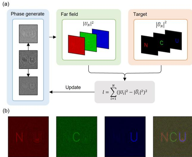
**Fig. 5.** Flowchart (a) and results (b) of multi-wavelength color metasurface holography
