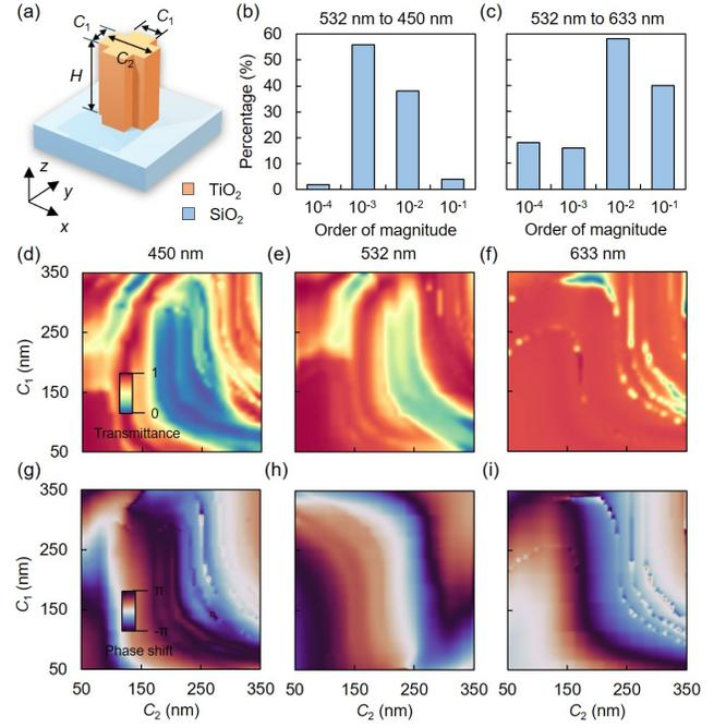
**Fig. 2.** The design of the metasurface. (a) Schematic of a single  $\text{TiO}_2$  meta-atom, where  $H = 800$  nm and  $P = 400$  nm (b, c) Fitting accuracy of the MLP model. (d-i) The simulated transmittance and phase shift of the meta-atom at wavelengths of 450, 532, and 633 nm, respectively.
