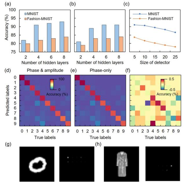
**Fig. 4.** Results of DW-MDNN. (a, b) Classification accuracy as a function of the number of hidden layers without and with phase correlation. (c) Classification accuracy as a function of the size of the detector. (d, e) Confusion matrix for amplitude crosstalk and phase-only (amplitude is considered to be a constant value). (f) Percentage error matrix between (d) and (e). (g, h) Predicted results of the network.
