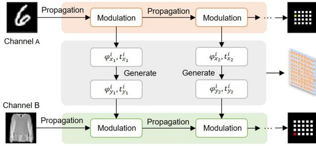
**Fig. 3.** The flowchart of DW-MDNN. The MNIST and Fashion-MNIST datasets are encoded into two independent channels, A and B. Incident light of different wavelengths passing through the same metasurface generates different transmission coefficients and phase shifts. The phase correlation method is introduced to establish a relationship between the phases of two channels.
