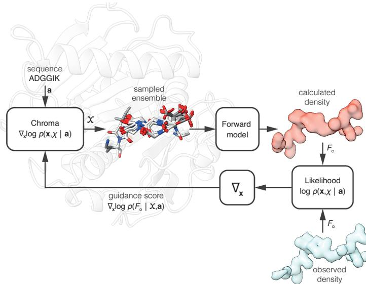
Figure 1: **The proposed density-guided protein ensemble generation method.** The diffusion model is used to sample a non-i.i.d. ensemble from which the likelihood of the observed electron density is calculated and used to guide the sampling.
