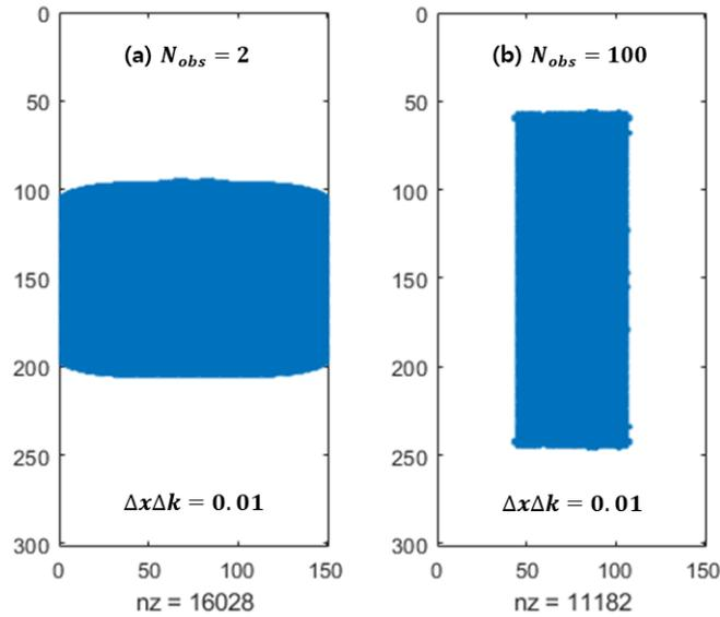
**Supplementary Material Figure 2 – The sparsity of the system matrix caused by nonlocal terms.**
