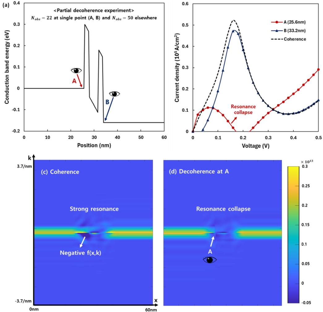
**Figure 4 – Partial decoherence experiment for resonant tunneling diode.**
