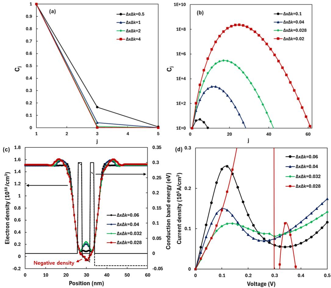
**Figure 2 – Numerical instability in cases of small mesh size.**
