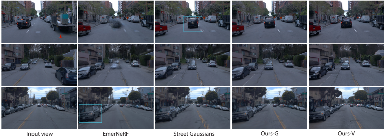
Figure 3. Qualitative comparisons on the Waymo [47] dataset. The camera is laterally shifted for 3 meters to left or right. Input view refers to the closest training camera. Ours-G denotes the dynamic 3DGS distilled from StreetCrafter and Ours-V denotes StreetCrafter.
