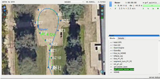
Figure 6: Screenshot from the Paparazzi’s GCS in simulation. Bézier points are represented as blue diamonds, while the desired trajectory is represented as a green line. The actual trajectory traced by the Rover is shown in blue.
