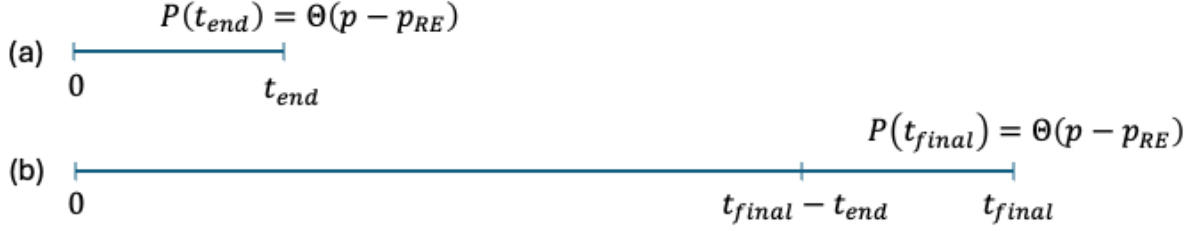
Figure 3. Panel (a) indicates an adjoint problem with the terminal condition P(t = t_{end}) = \Theta(p - p_{RE}) , and Eq. (5) is integrated backward to t = 0 . The solution to this problem will be identical to a problem with the terminal condition at P(t = t_{final}) = \Theta(p - p_{RE}) and integrating backward until t = t_{final} - t_{end} .
