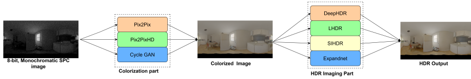
Fig. 2: This study examines various methods for converting a monochromatic SPC image to a Color HDR image using state-of-the-art techniques. We explore Pix2Pix, Pix2PixHD, and CycleGAN for the translation from monochromatic to color. Subsequently, we investigate DeepHDR, LHDR, SIHDR, and ExpandNet for converting the colorized image to its HDR version.
