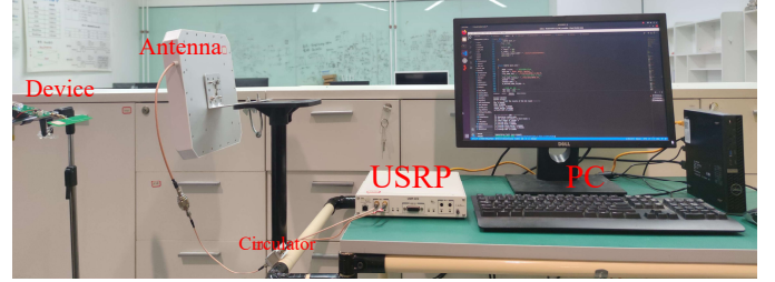
Fig. 2. Illustrating of an A-IoT demonstration system.
