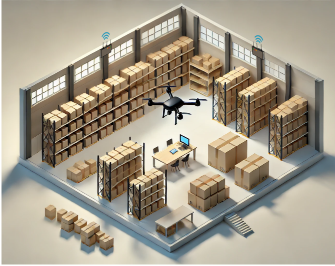
Fig. 1: Illustration of an indoor warehouse environment where a drone navigates while two 5G base stations provide Time-of-Arrival (ToA) measurements. The base stations assist in refining the drone’s positional accuracy, supporting real-time localization and mapping (The warehouse figure was generated using OpenAI’s ChatGPT).
