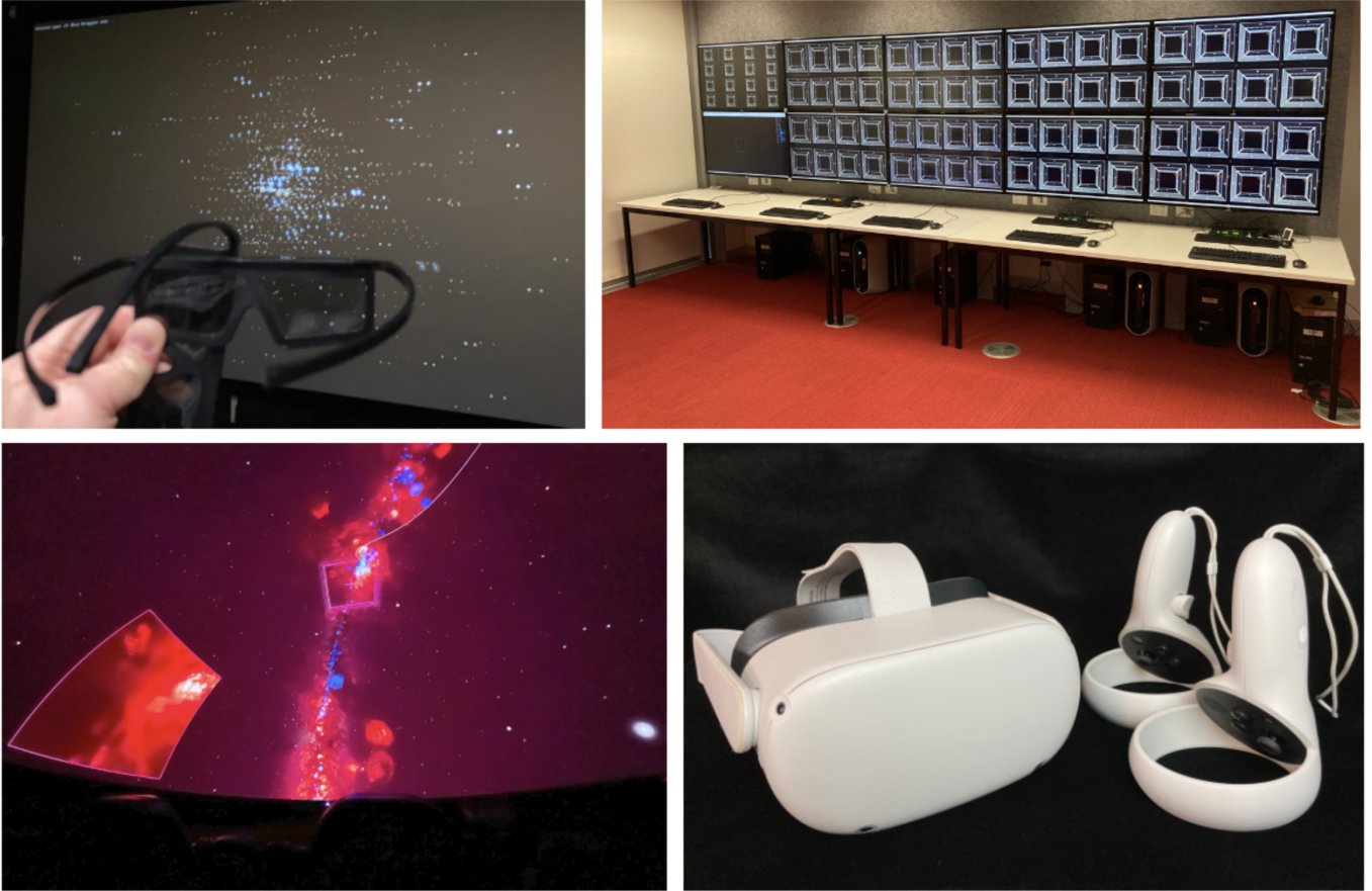
Figure 1: Examples of the four advanced image displays that continue to be the front runners for wider-scale adoption in astronomy and astrophysics research. (Top left) Large-format stereoscopic projection using a two-projector set-up with linear polarising filters and polarisation-preserving silver screen (globular cluster simulation by J. Hurley, visualisation by D. Barnes). (Top right) The Swinburne Discovery Wall is a tiled display wall comprising a matrix of ten 4K UHD displays for a total 84 million pixels, described in (Fluke et al., 2023). (Bottom left) Visualisation of the local Milky Way projected onto the dome of the Hayden Planetarium (American Museum of Natural History). (Bottom right) The Meta Quest 2 virtual reality head-mounted display with handheld controllers. The image of the Hayden Planetarium is courtesy A.Goodman and J.Faherty (see http://milkyway3d.org for details). The other images are the work of C.Fluke (CC-BY-NC).
