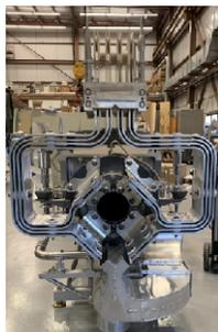
FIG. 3. An image of the horn 1 showing the air diverter at the bottom as the upgraded cooling system to the horn striplines.
