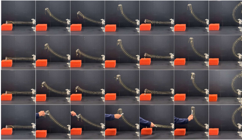
Figure 14: Snapshots of the TDCR under sliding mode control: First row shows normal conditions, second row with a 20 g weight hanging from the tip, third row with a 50 g weight, and fourth row under random impact disturbances
