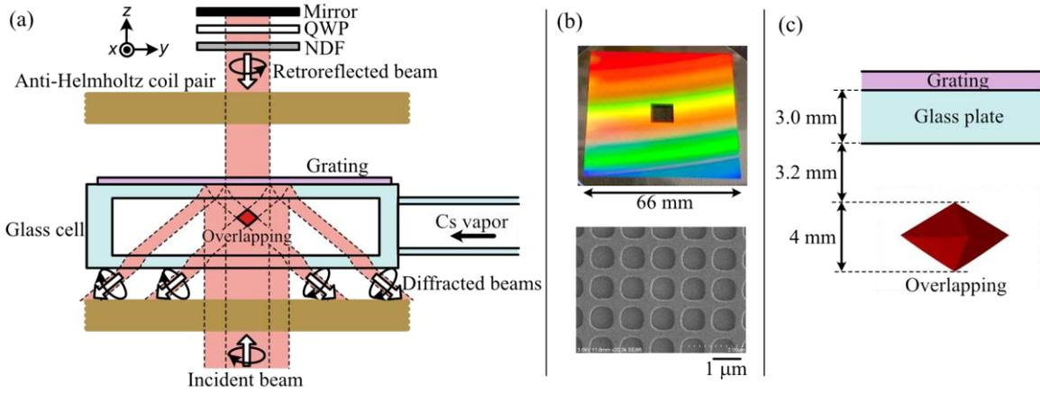
Fig. 1 (a) Side view of the experimental setup of the balanced gMOT. The orthogonal coordinate system is also indicated. The sides of the grating are parallel to the  $x$ - or  $y$ -axis. (b) (Top) Photograph of the 2D grating with an aperture. (Bottom) Electron microscopy image of the dot-shaped microstructure on the 2D grating. (c) Three-dimensional view of the overlapping region from the horizontal direction at an angle of  $30^\circ$  to the  $x$ -axis.
