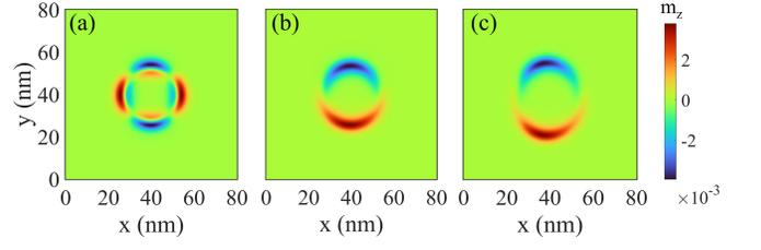
FIG. 3. Out-of-plane magnetization of: (a) Stationary skyrmion, and (b) and (c) moving skyrmions at  $u = u' = 5.2\text{ m/s}$  and  $u = u' = 8\text{ m/s}$ , respectively. The charge current is applied in the  $y$ -direction. Parameters used:  $\alpha = 0.01$ ,  $\beta = 0.01$ ,  $H_{\text{an}} = 0.22\text{ T}$ ,  $M_s = 1.3 \times 10^2\text{ kA/m}$ ,  $D = 0.55\text{ mJ/m}^2$ .
