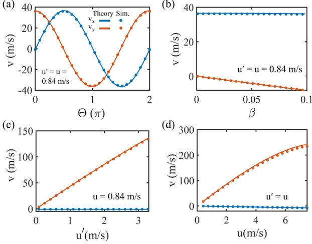
FIG. 4. Components of the skyrmion velocity,  $v_x$  and  $v_y$ , calculated from micromagnetics and from Eqs. (21) and (22) for different directions of the charge current with respect to crystallographic axes described by  $\Theta$ . Parameters used:  $\alpha = 0.01$ ,  $\beta = 0.01$  (in (a), (c), and (d)),  $H_{an} = 0.22$  T,  $M_s = 1.3 \times 10^2$  kA/m,  $D = 0.55$  mJ/m<sup>2</sup>. The current is applied in the  $x$ -direction ( $\Theta = 0$ ) in (b)-(d).
