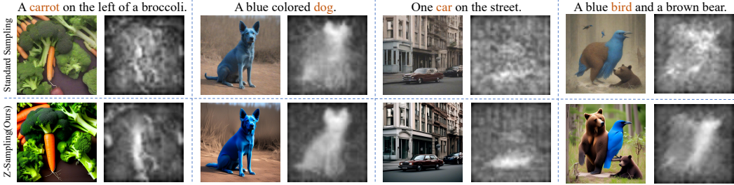
Figure 5: The cross-attention map highlights the interaction between the entity token (red color) and latent variables. Z-Sampling optimizes the latent so that it is more suitable for generating concepts in the related-prompt. For example, in the zigzag path of the second column, semantically injected latents exhibit sharper attention on “dog” with relatively clear boundaries.
