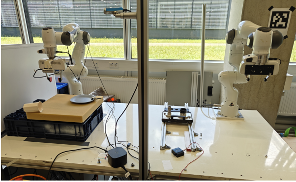
Fig. 7. Robotic experimental setup consisting of 2 Franka Emika Panda robot arms for teleoperation and an over-the-shoulder camera (Realsense d435). The left arm is follower robot, while the right one acts as the leader . During the teaching phase, a human expert controls the leader arm to send the desired reference to the follower robot via ROS. During testing, only the follower arm is operational.
