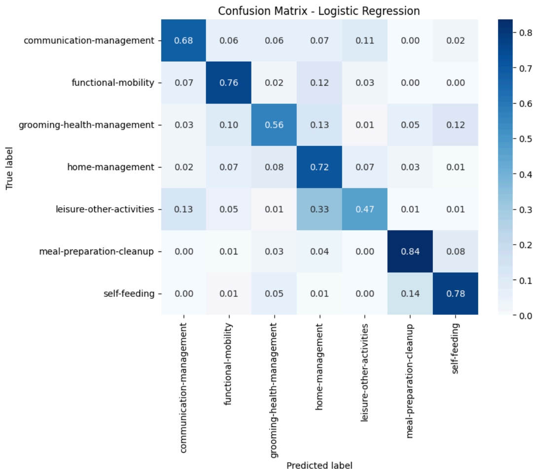
Figure 2: Confusion matrix for LR using binary presence feature vector with active objects.
