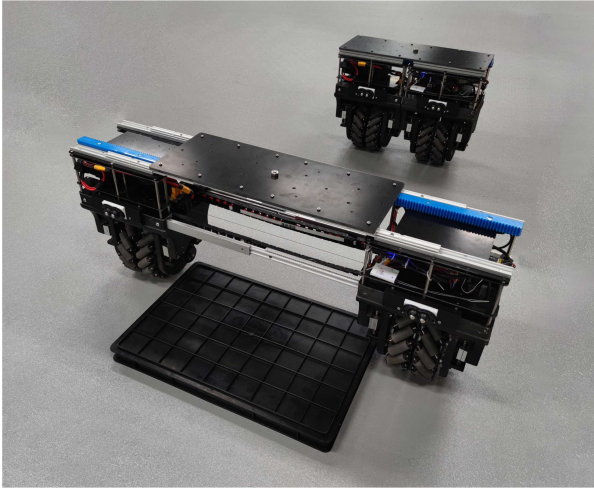
Fig. 1. Proposed Prototype which can simultaneous reconfigure and omnidirectional mobile using the Omni Differential Drive (ODD).
